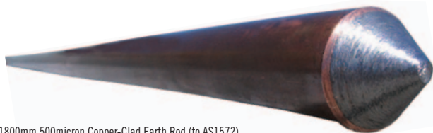
12mm 1800mm 500micron Copper-Clad Earth Rod (to AS1572)
