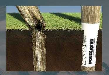
Using Polesaver sleeves to prevent ground rot is a safe and simple economic way of extending the lifetime of treated soft wood and hardwood poles. Polesaver patented sleeves are non-toxic and quickly and easily applied to the treated poles using heat. Polesaver sleeves can be used on both new poles and retrofitted to sound poles in service providing a long lasting, tough and durable barrier to the causes of ground rot and decay.
