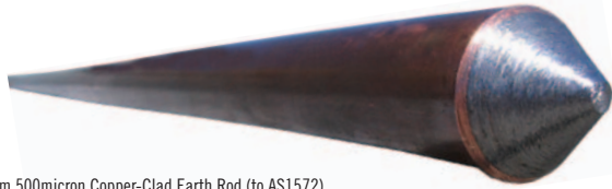
12.8mm 1800mm 500micron Copper-Clad Earth Rod (to AS1572)
